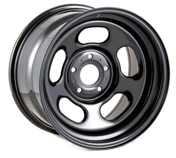
Also new from Rugged Ridge are these Trail Runner classic steel wheels. These, like the Jeeps they're made to go on, are genyooine Yankee products, and they're built tough. They're also built to the latest standards and have a hub-centric design so the wheel is precisely centred which helps reduce any vibration.
